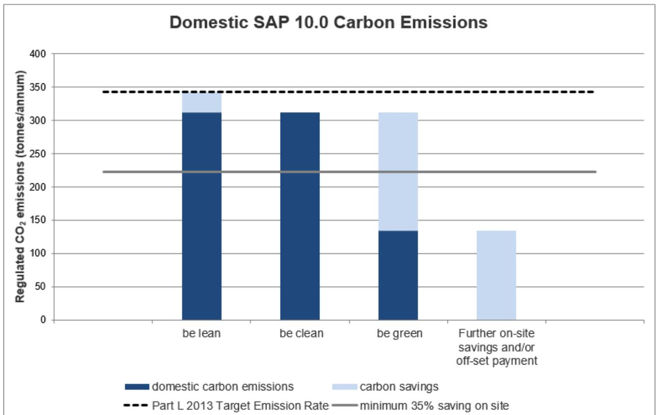
The recommended approach for adhering to London Plan targets for FDS is a combination of 'Be Lean', 'Be Clean', 'Be Green' and 'Be Seen' measures. 'Be Seen' measures are not calculated.
