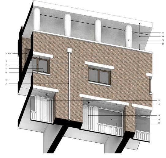
Cutaway isometric bay study
