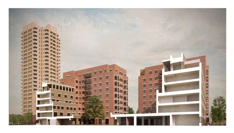
Perspective section C: The grade level courtyard provides a secure route through the block between Thurlow Street and Alvey Street, from which secure bicycle storage is easily accessible. Location of cycle storage and ancillary frontage in this location allows for continuous active frontage to the street facing sides of the block.
