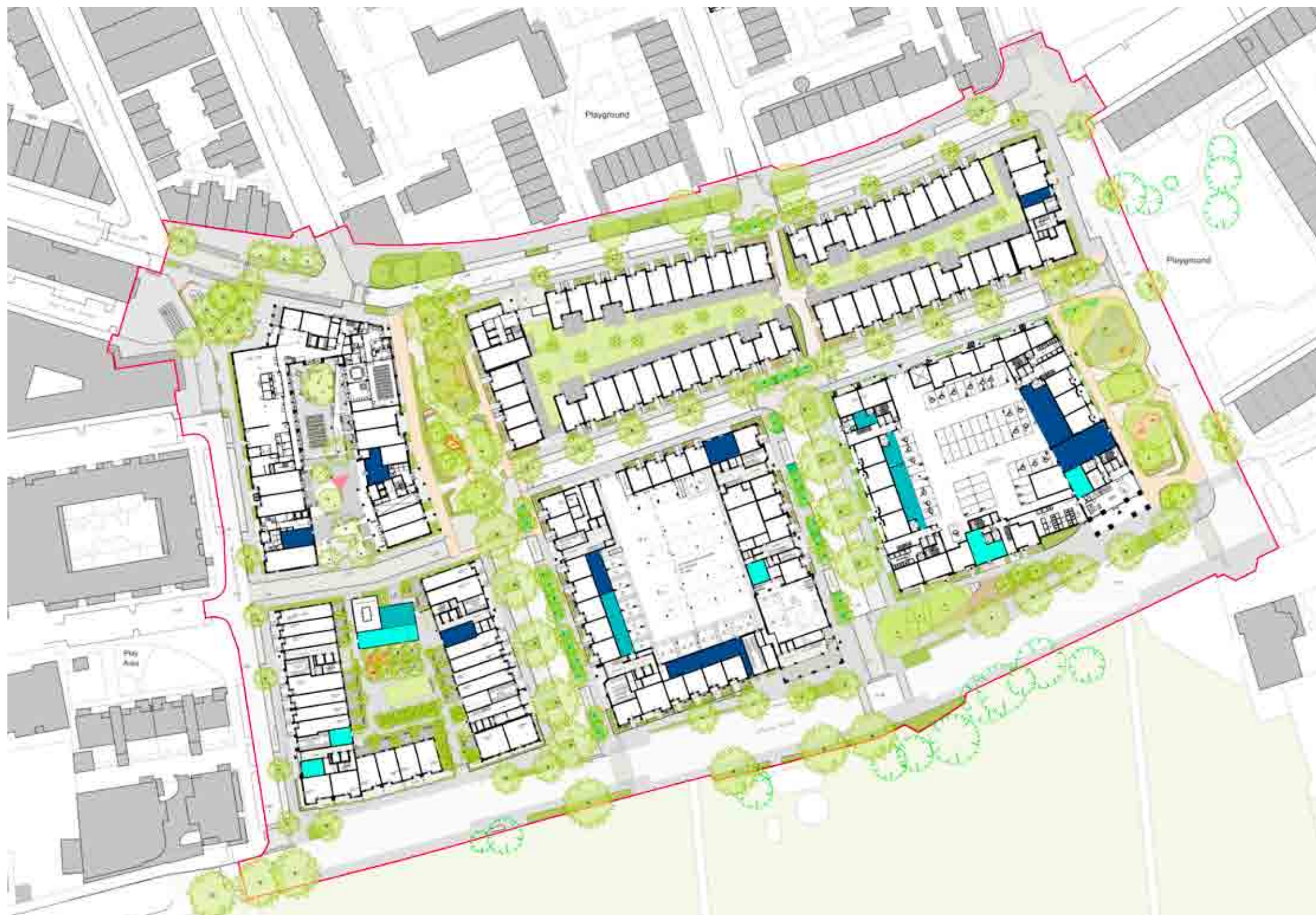
Fig 4.72 Sitewide ground floor plan showing location of cycle storage across FDS.
