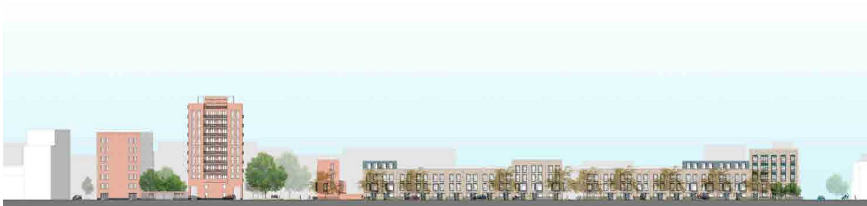
Fig 2.6 South elevation/ north side of East West street showing how lower massing presents a more continuous frontage comprising terraced houses and smaller mansion blocks more reminiscent of the conservation area to the north of the site.
