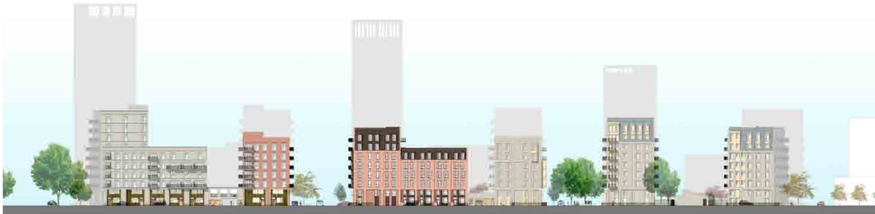
Fig 2.5 East West route proposed north elevation/ south side of street showing how taller elevation comprises a series of connected and stand alone mansion blocks.
