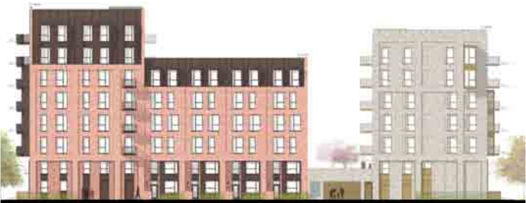
Fig 2.8 Block 5C showing mansard roof to upper storeys to reduce apparent mass and height of elevation by creating a lower parapet shoulder height.
